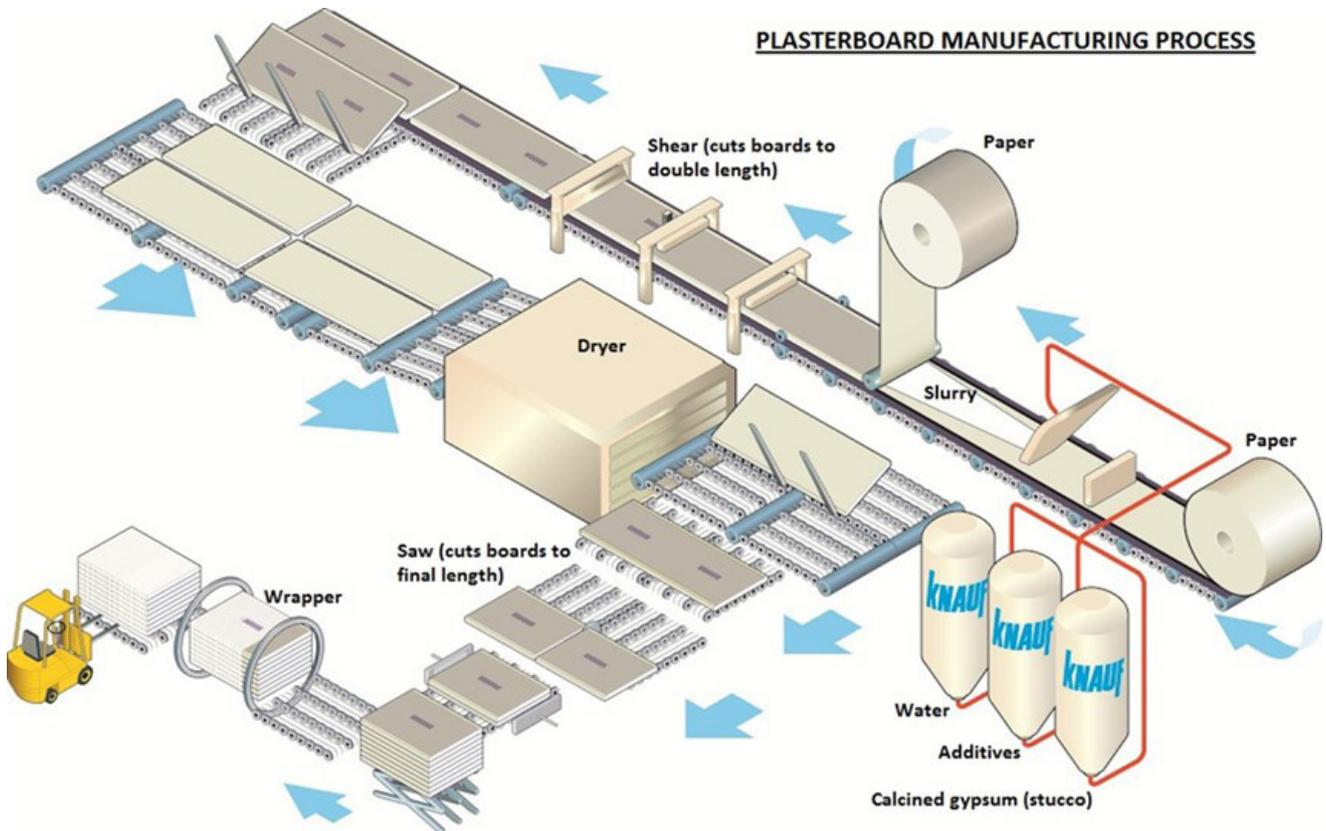
Raw materials are homogeneously mixed to form a gypsum slurry that is spread via hose outlets onto a paper liner on a moving belt conveyor. A second paper line is fed onto the production line from above to form the plasterboard. The plasterboard continues along the production line where it is finished, dried and cut to size.
