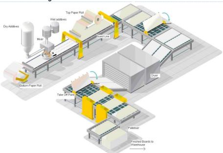
The initial materials are homogenously mixed to form a gypsum slurry that is spread via hose outlets onto a paper liner on a moving belt conveyor. A second paper liner is fed onto the production line from above to form the plasterboard. The plasterboard continues along the production line where it is finished, dried, and cut to size.
