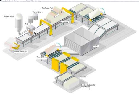
The initial materials are homogenously mixed to form a gypsum slurry that is spread via hose outlets onto a glass fiber mat on a moving belt conveyor. A second glass fiber mat is fed onto the production line from above to form the plasterboard. The plasterboard continues along the production line where it is finished, dried, and cut to size.
